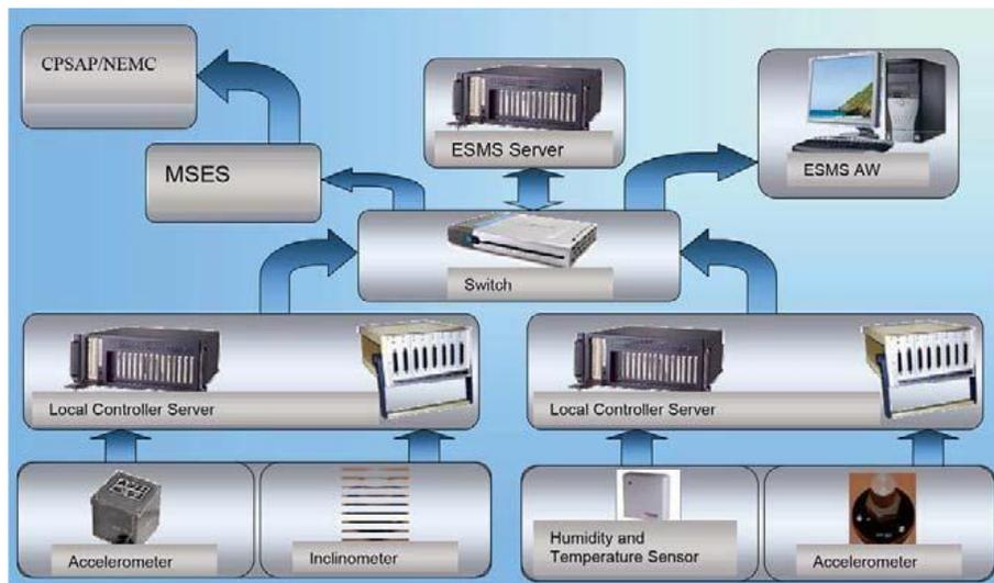
The ESMS is comprised by equipment for monitoring changes in the condition of foundations and engineering structures of buildings and constructions; engineering protection facilities, and also, if there is any corresponding hazard, for monitoring the areas of possible mudflows, mudslides and avalanches in the building or construction operation area. It includes:
